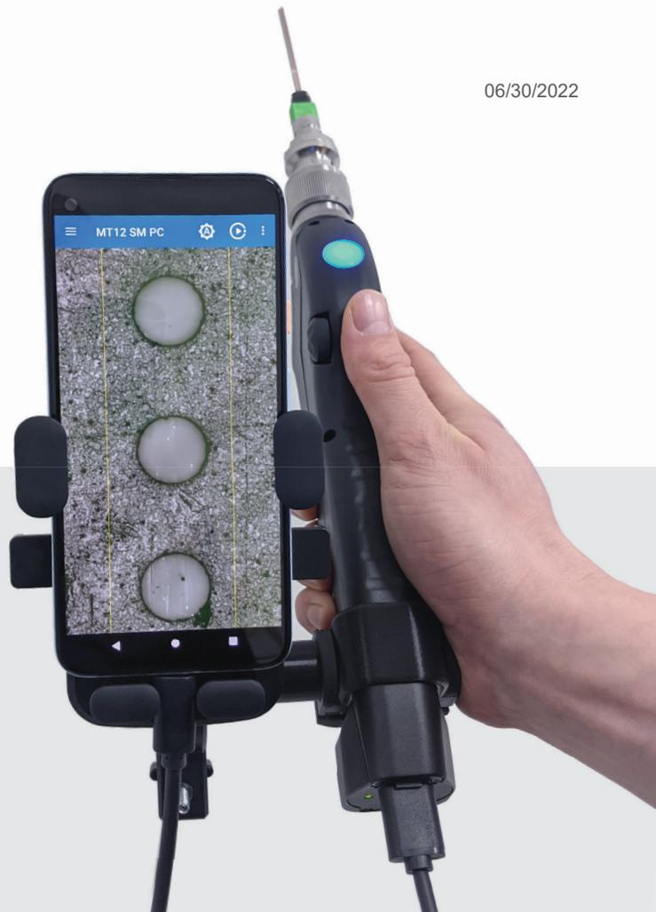
Handy, fast, automated inspection tool for data-centers, fiber-to-the-antenna and other field applications. Single and multi-fiber patch cords, bulkhead and QSFP modules – all inspected with the unsurpassed resolution and level of detail.
